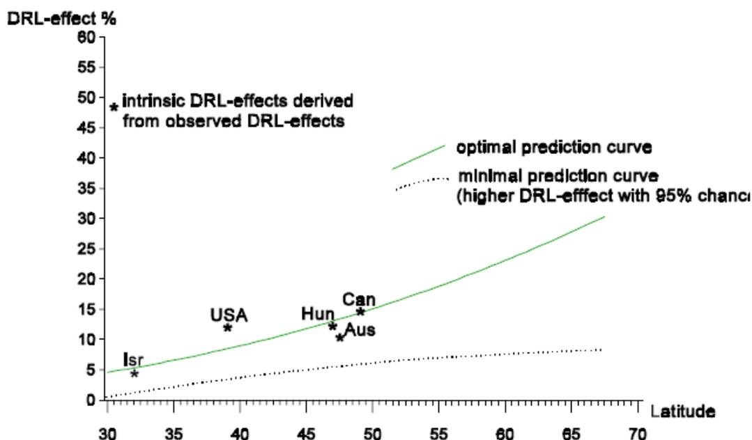
Figure 2.1: Prediction curves for intrinsic effects of DRL on all multi-party daytime accidents in different countries: an optimal and a minimum prediction curves (with a 95% confidence interval). Source: Koornstra et al (1997).
